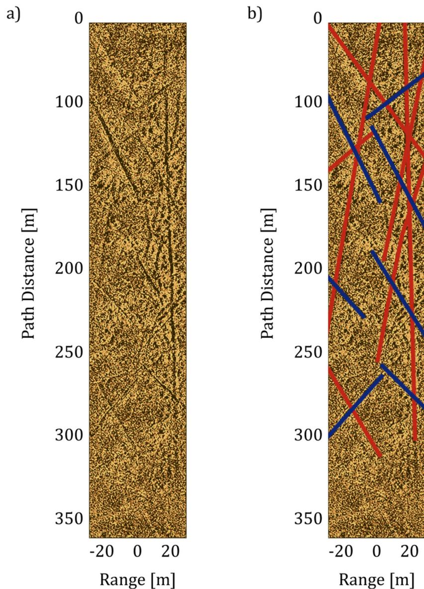
**Fig. 11.** Examples of high resolution (900 kHz frequency) side-scan sonar images of sea bottom with visible trawl marks. Post processing was performed for better visualisation. Colour-marked lines present supposed generations of scars (b) – younger as blue and older as red. The images were obtained near the Bornholm dumpsite at 55°19.2'N, 15°37.6'E. (For interpretation of the references to colour in this figure legend, the reader is referred to the web version of this article.)
